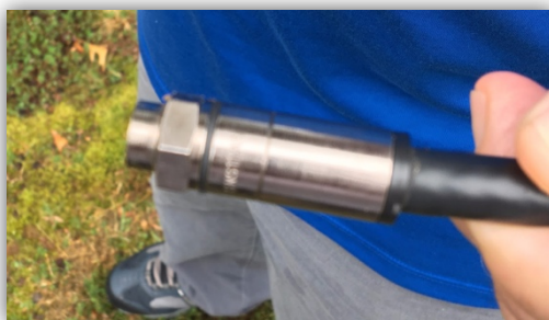
Figure 32: Bad Compression Type F-Connector
