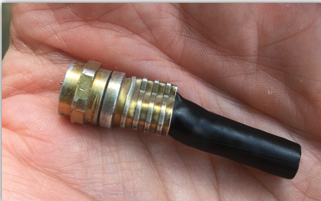
Figure 18: Crimp-on F-connector On Back of Modem Causing Micro-Reflection
