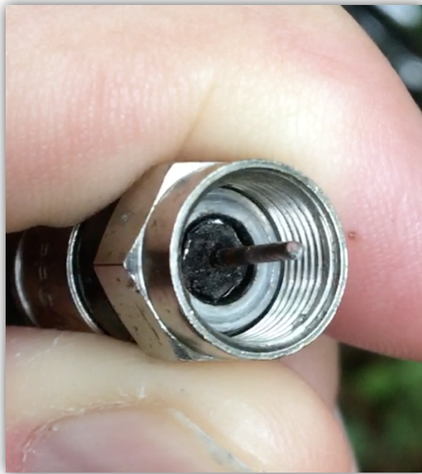
Figure 21: Blackening of Center Conductor and Insulating Dielectric Indicating Possible Surge
