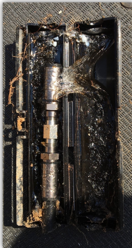
Figure 11: Opened Splice Enclosure with Water Ingress and Corrosion
