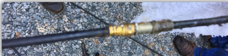
Figure 5: Crimp-on F-Connectors Exposed to Water and Corroded
