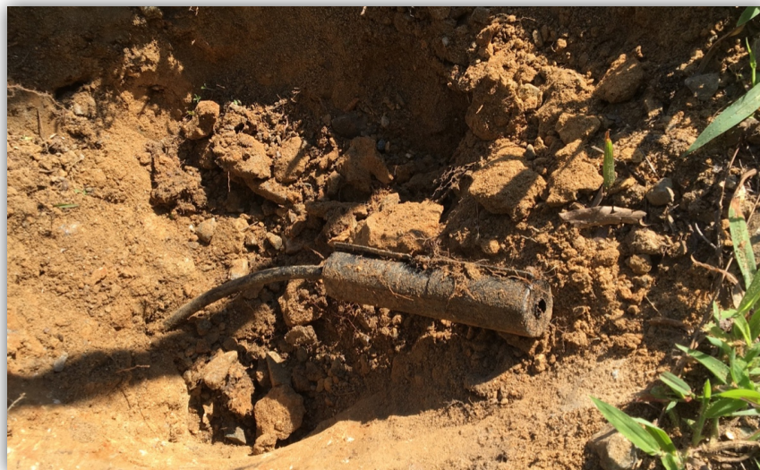
Figure 10: Buried Splice Enclosure with Series 11 Cable Pulled from F-Connector
